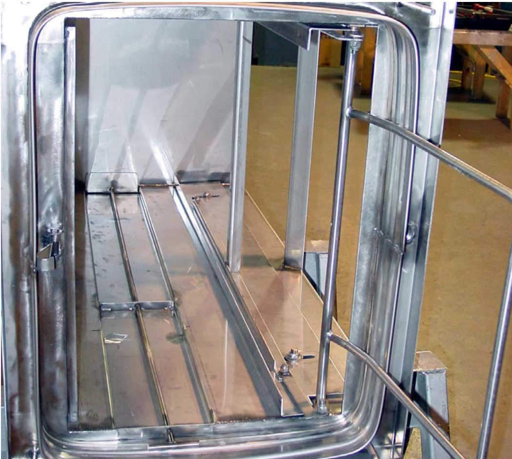
Locking arm of gel seal housing Figure 1-2
